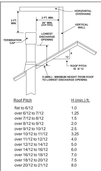
Figure 31. Minimum Height from Roof to Lowest Discharge Opening
